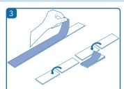
Remove the back lining from the adhesive pad and stick 2 pads together (x2).
