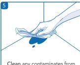
Clean any contaminates from the installation surface with the alcohol wipe.
