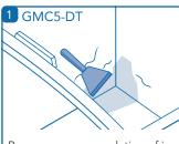
Remove any accumulation of ice from the mounting surface
